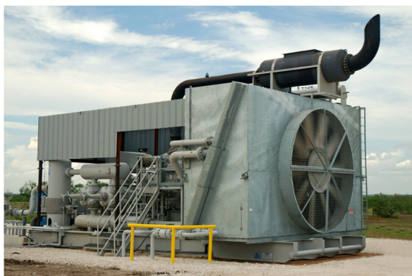
Gas Pipeline Compressor
